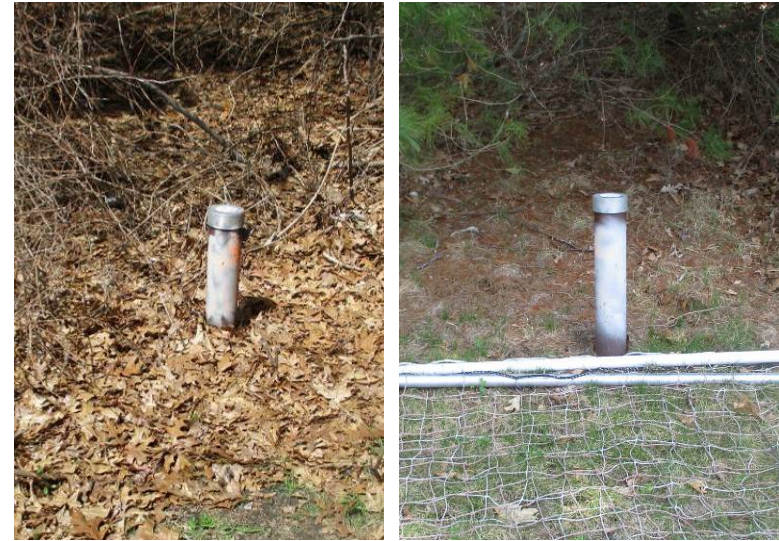
Several down-field testing wells located at various points around the property are utilized to monitor effluent levels, soil absorption efficiency, and ensure that the post-treated water emanating from the field meets local standards.
