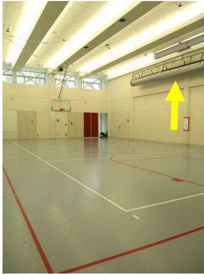
Gym 3 features a single basketball court with painted synthetic surface and a cable-supported wrestling mat storage system (arrow).
